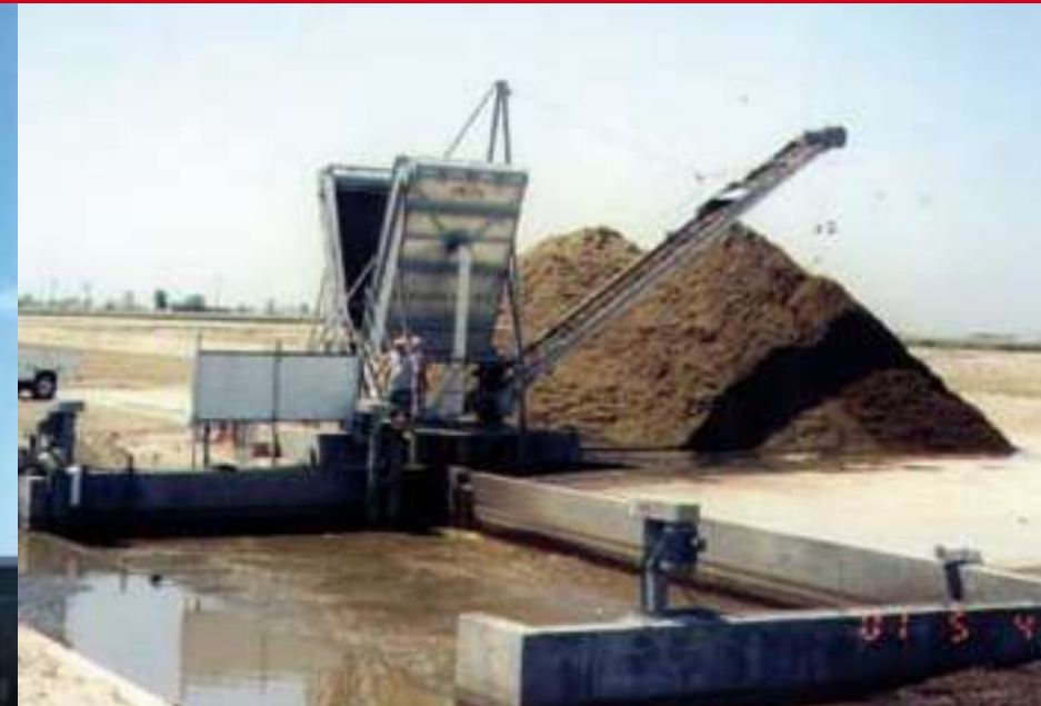
SLOPED SCREEN WITH STRUCTURE - NO MOVING PARTS
